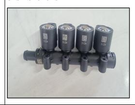
Gas injectors are vital components in modern fuel injection systems. They precisely deliver required quantity of fuel into the engine manifold, optimizing engine performance, fuel efficiency, and emissions. There are various types of gas injectors, including port and direct injection. Regular maintenance is essential to ensure their proper functioning and long-lasting performance.
