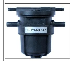
Filter with PT/MAP Sensor is a combination device that integrates a filter element with a pressure sensor. It's used in engine management systems to accurately measure and control intake manifold pressure. The filter ensures clean air for the sensor, leading to accurate readings, improved engine performance, emissions control, and sensor protection.
