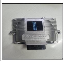
The C-OBDII-4 Cyl ECU and wiring harness are essential components in four-cylinder vehicles. The ECU ensures emissions compliance, optimizes performance, and facilitates diagnostics. The wiring harness connects the ECU to various sensors and actuators, enabling data transmission and control. Together, they play a crucial role in modern vehicles, ensuring efficient operation and compliance with environmental regulations.
